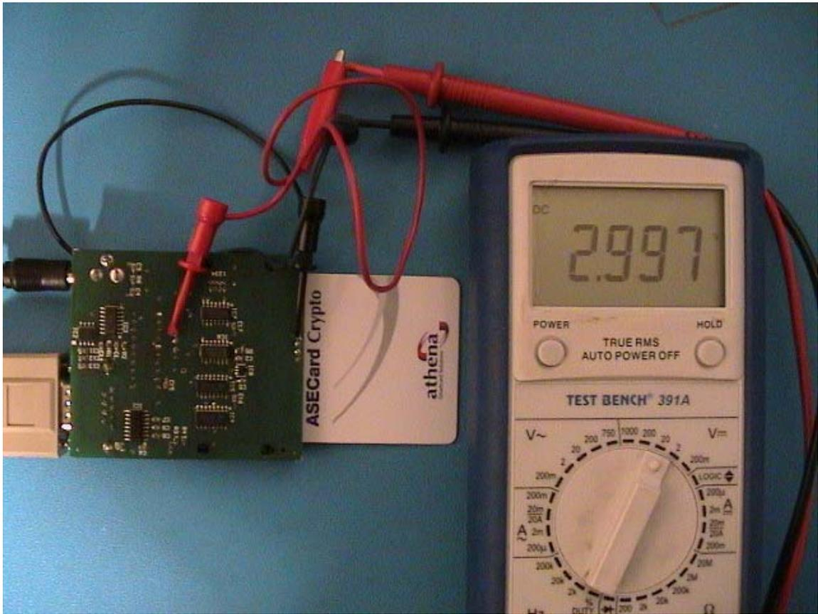
**Figure 3:** Bottom view of ASECard Crypto ISO7816 Class B smart card in Whiteviper unloader running iso7816\_vcc. The digital multimeter is displaying the DC voltage being supplied between the VCC and GND contacts of the smart card slot.
