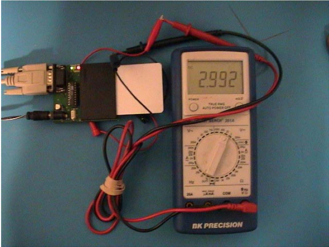
**Figure 2:** Top view of ASECard Crypto ISO 7816 Class B smart card in Whiteviper unlooper running iso7816\_vcc. The digital multimeter is displaying the DC voltage being supplied across the VCC and GND contacts of the smart card slot.
