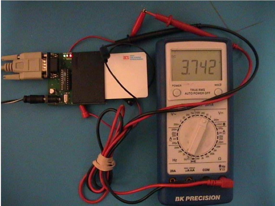
**Figure 1:** ACOS1 8K ISO 7816 smart card in Whiteviper unlooper running iso7816\_vcc. The digital multimeter is displaying the DC voltage being supplied across the VCC and GND contacts of the smart card slot.
